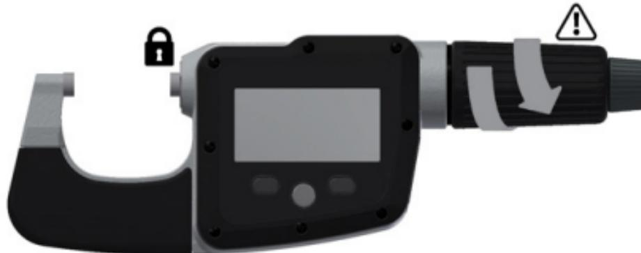
To unlock the spindle, rotate the speeder to extend the spindle, regaining control via the thimble.
